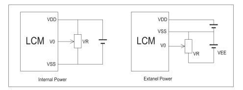
$V_{DD-}V_0$ : LCD Driving voltage VR: 10k~20k
